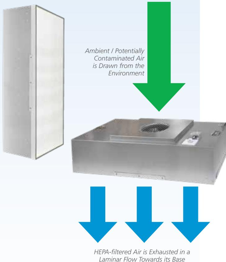
**Esco Airstream® Fan Filter Units (FFUs).** All TTC Schemes can be integrated with FFUs. It is designed to draw in ambient air from the top of the module, and supply clean filtered air vertically in a unidirectional (laminar) air stream toward a dedicated area or space.
